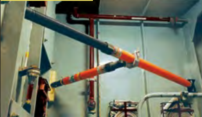
H-Type, can be used vertically or horizontally and takes moderate pressure (see table) as the pressure acts perpendicular to the load axis.
