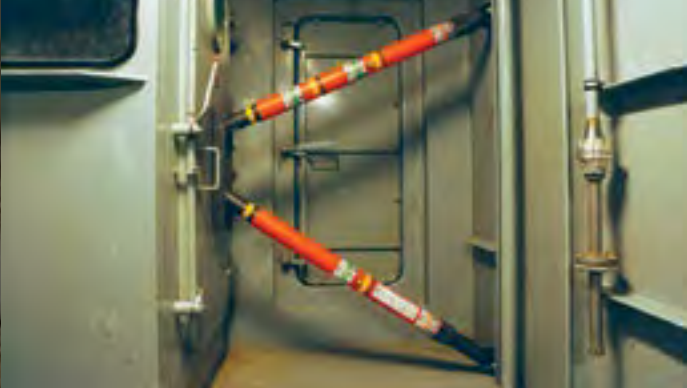
K-Type, can be used vertically or horizontally and takes full pressure (see table) as the pressure acts parallel to the load axis.
